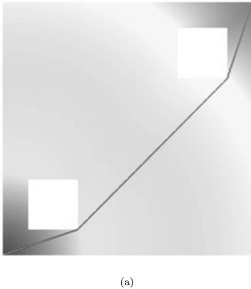
Fig. 6 Geodesic distance on a planar mesh with a hole
