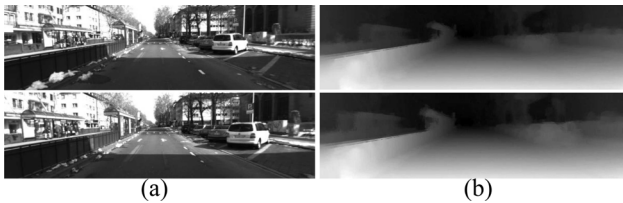
Figure 3: Our inference disparity map from Karlsruhe dataset. (a) Left frame from stereo video. (b) Inference results of the proposed approach.
