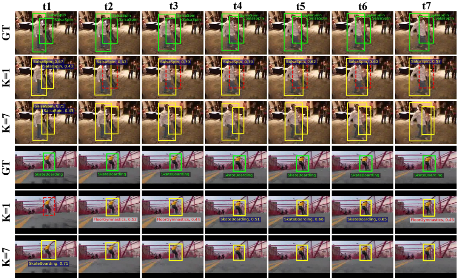
Fig. 5. Examples of Per-frame (K=1) and Tubelet (K=7) Detection. The yellow color boxes present detection results, whose categories and scores are provided beside. Yellow boxes categories represent classifying correctly and red ones represent wrong. Red dashed boxes represent missed actors. Green boxes and categories are the ground truth. As our MOC-detector generates only one score and category for one tubelet, the score and category are only presented in the first frame for tubelet (K=7) detection. Note that we set the visualization threshold as 0.4.
