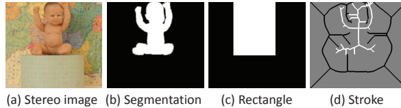
Fig. 5. Input types. For both rectangle and stroke input, the white pixels indicate “Object” and black ones indicate “Background”.
