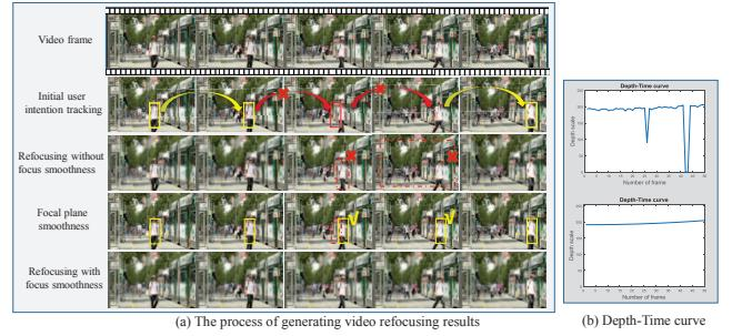
**Fig. 4.** The comparison between video refocusing without and with focal smoothness, (a) illustrates the initial tracking results of user intention and the improved effects by utilizing focal plane smoothness, red rectangle means missing match while yellow is the correct tracking results, and (b) is the depth-time curve before and after focal plane smoothness.
