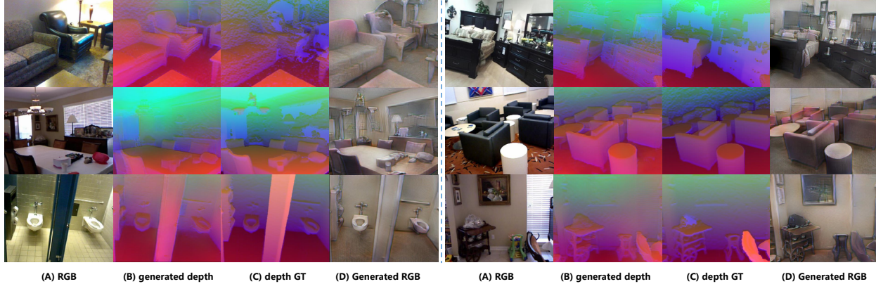
Figure 6. Examples of generated data by our TrecgNet from test set of SUN RGB-D dataset. (B) are depth images translated from original RGB data (A), and (D) are generated RGB images using original depth ones (C).
